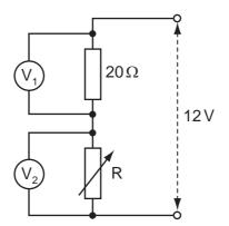
When R has a value of  $20\Omega$ , the voltmeter readings are equal.
