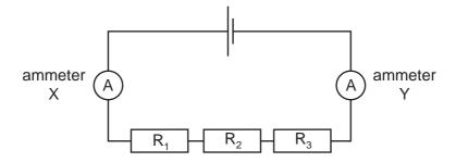
Which of the ammeters will show the current in resistor R<sub>2</sub>?
