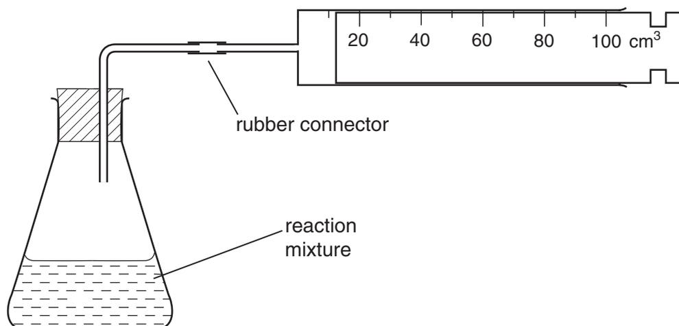
By using a measuring cylinder, 20 cm<sup>3</sup> of hydrogen peroxide was placed in the flask and 0.8 g of the catalyst, manganese(IV) oxide was added. The bung was replaced and the gas collected was measured at 1 minute intervals. The results were plotted on the grid (opposite).
